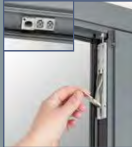
Concealed shoot bolts at the top and bottom of the inactive leaf hold the door securely in place. The adjustable keeps allow for easy alignment of the leaf position for a precise fit.
